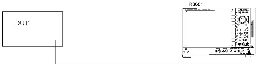
Figure 4-24 Connection Diagram for the Modulation Analysis that Uses the Multi Frame Mode
