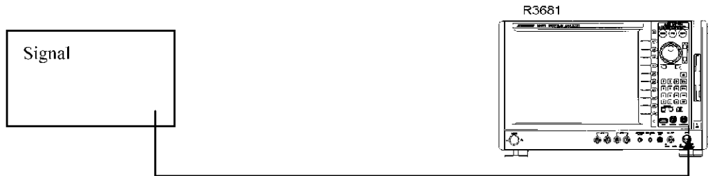
Figure 4-8 Connection Diagram for the Modulation Analysis that Uses the Single Frame Mode
