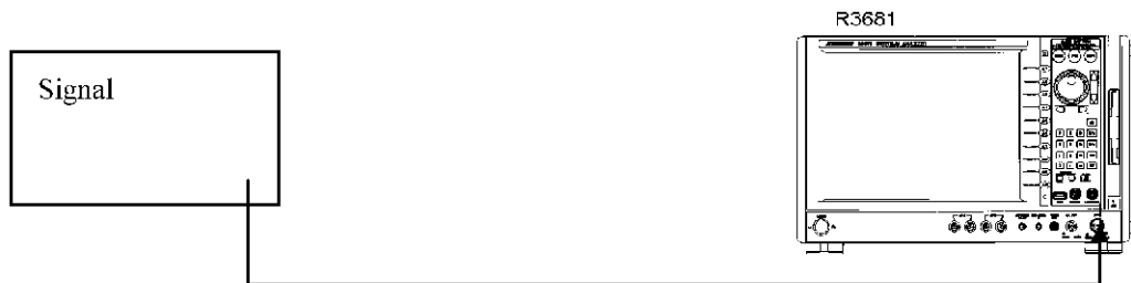
Figure 4-1 Connection Diagram for the Modulation Analysis that Uses the Multi Frame Mode
